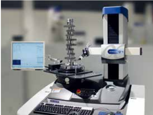
Measuring crankshaft using designated jig tool
