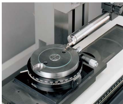
Measurement of hard disk using SURFCOM 480A
