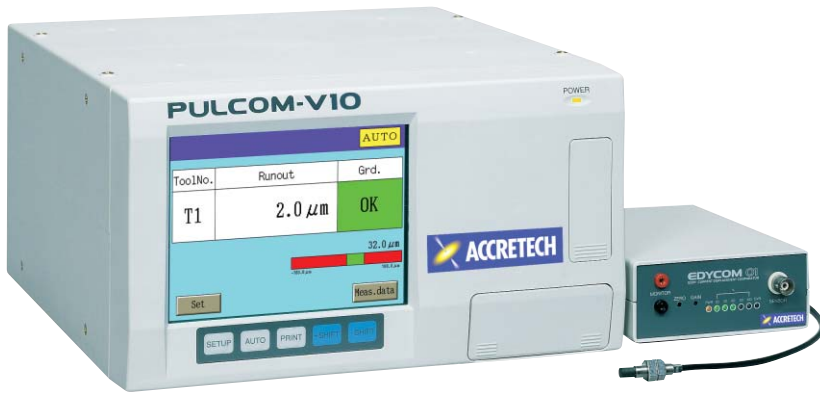
ATC Run-Out Detection Improper chucking caused by chips or other foreign matter in the tool chuck is detected by run-out of the shank flange.
